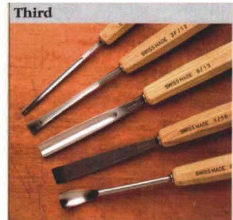
5mm No. 5 12mm No. 3 fishtail 13mm No. 8 16mm No. 1 16mm No. 8 spoon
